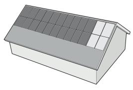
7.2 kW package installed on roof where you have decided not to install e.g. two panels (6.5 kW).
