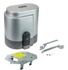
ESM6 ACTO 2200A non-reversible 230 V~ electromechanical operator for sliding gates up to 2200 kg, tertiary and industrial use, electronic control card, 433 MHz radio receiver, optical encoder, electromechanical limit switches, complete with transformer, fixing plate
